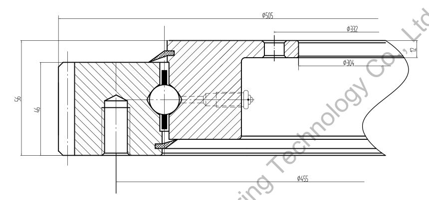
Modulem5Number of teethz99Addendum modificationx0Pressure anglea20°Accuracy grade10-ISO 1328/97
